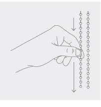
Repeat step 2 pulling chain in the opposite direction until travellers are fully aligned.
