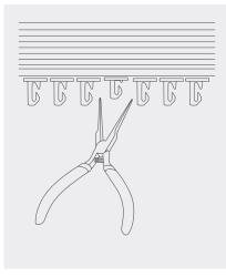
the headrail have been pushed in, if they have, using a pair of pliers, gently pull the pegs back out.
