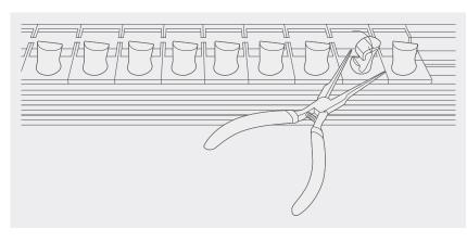
Did this align all the pegs? If not, gently rotate the lazy traveller with a pair of pliers. The traveller will then click into place accordingly.
