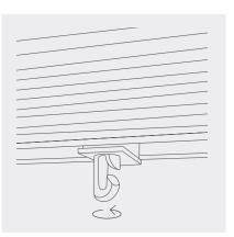
Do runners rotate normally? If yes, return the runners to the open position and add the louvres.
